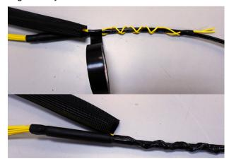
**Step 4:** Pull back the Techflex to insert the connectors.
