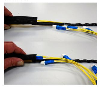
**Step 5:** Bring the Techflex over the legs and wrap with electrician tape.
